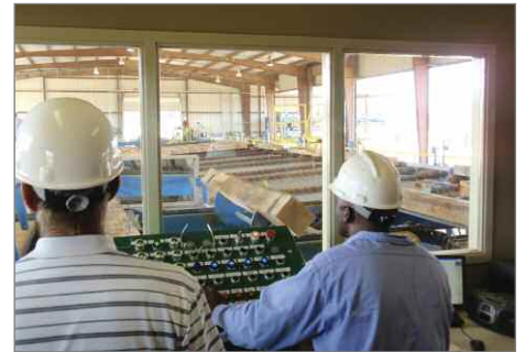
After a safety briefing, the tour started in possibly the most spacious and comfortable tie grading booth in the industry which, for many reasons—not the least of which is safety—offers the grader a panoramic view of the entire grading, incising and end-planting operation.
