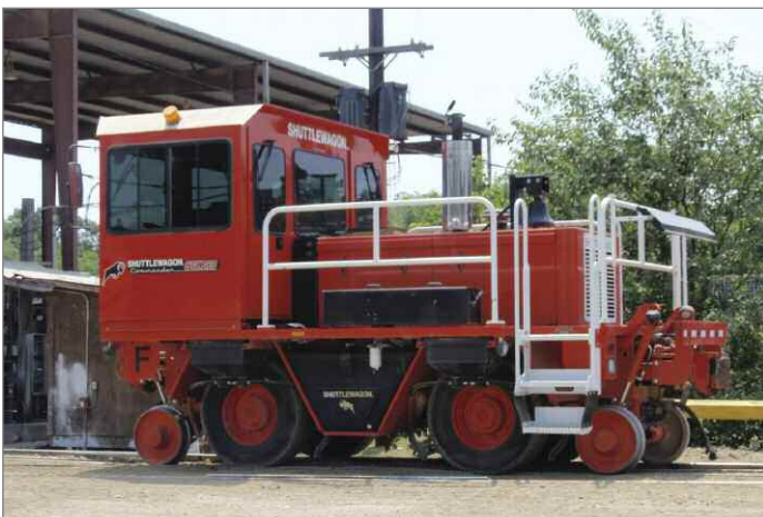
Two unique pieces of equipment are pictured here. The Shuttlewagon (left), which can maneuver up to 15 fully loaded gondola cars around the facility, and this Fuchs piece (right), capable of loading a full bundle of treated ties into a railcar in one bite, were the talk of the stop.
