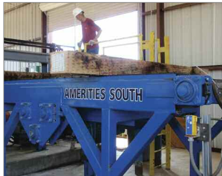
On the other end of the building, P&G Manufacturing's newest end-plater readies the ties for the air-drying yard.
